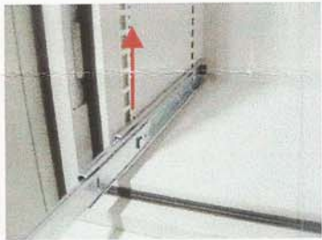
③ Lift front hook upward.
